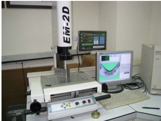
Fig. 3 The performance characteristics were measurement by the vision measuring machine (Mimn Tay EM-2D)
