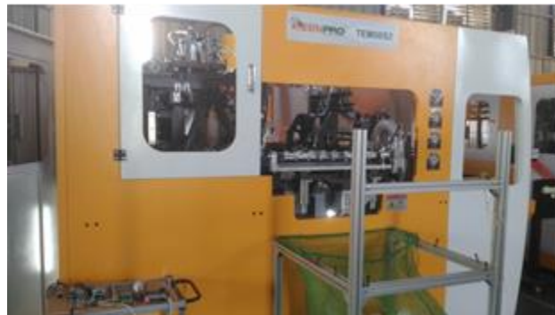
Fig. 1. The blow molding machine typed of EM08S1 by the KEENPRO Precision Industry Corp [9].
